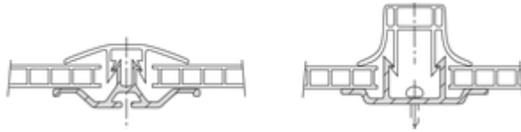
Figure 2. Depiction of Typical Two-Part Plastic and Metal Connecting Profiles Currently Used
